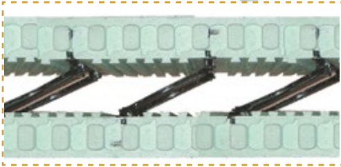
Close view of folding metal-hinged web
