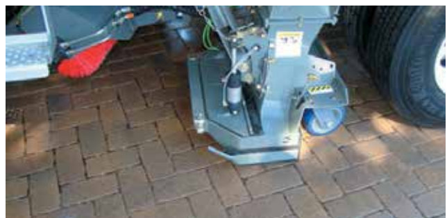
Vacuum truck for restorative maintenance
